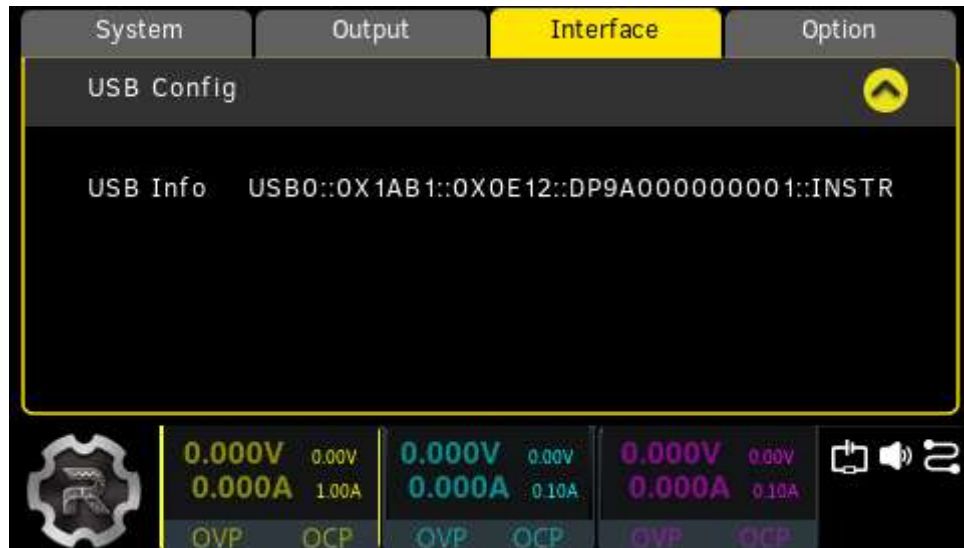
Figure 13.8 USB Configuration Interface
