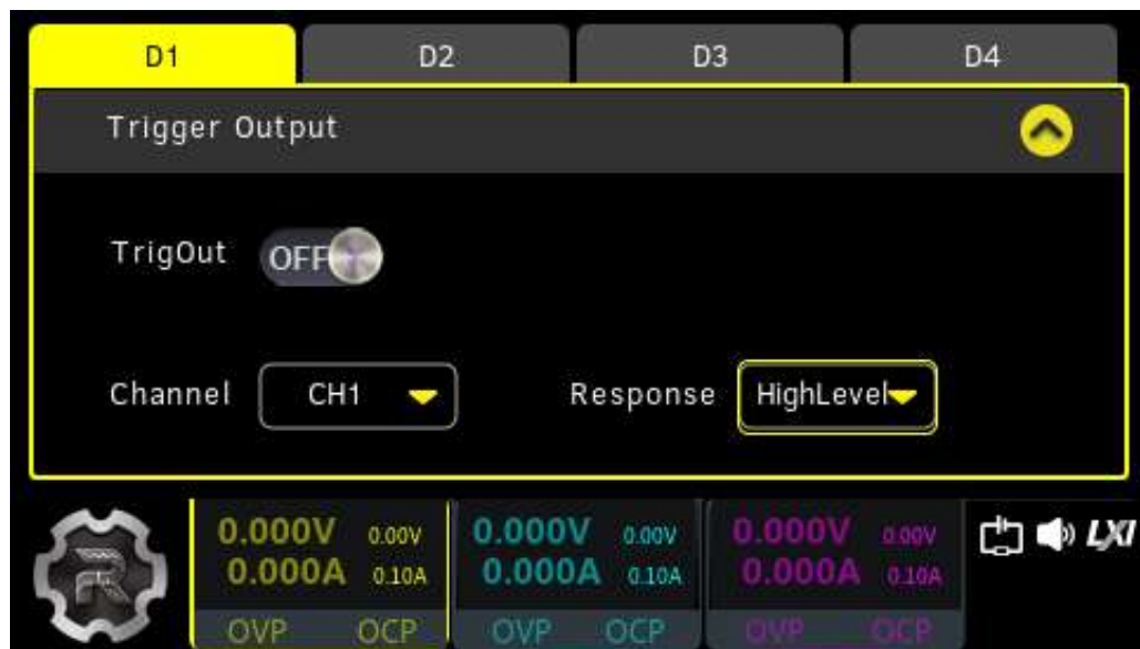
Figure 11.4 Trigger Output Setting Interface
