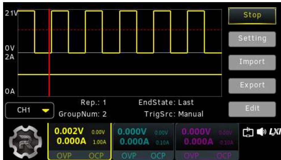
Figure 9.5 Arb Output Interface
