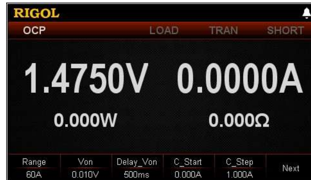
Figure 2-30 Main Interface of OCP Test Function
