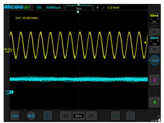
High frequency AC/DC current probe can easily measure signals over 20MHz (Yellow waveform on CH1)
