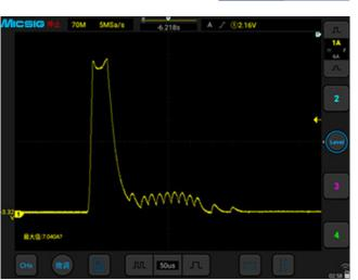
Surge current waveform at power adapter startup
